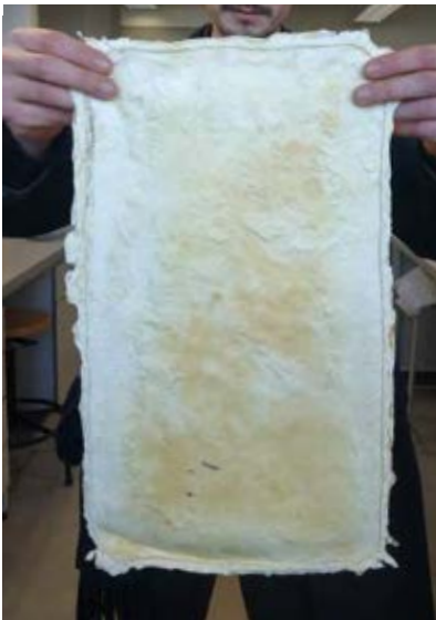
Production and process of mycelium leather, ELSACKER Elise & VANDELOOK Simon (VUB) - From left to right : Fig.27 - A 35 x 50cm mycelium leather ... Fig.28 which is then decomposed into few steps, showing the generation AND, because of the living aspect, the regeneration of a damaged mycelium based leather
