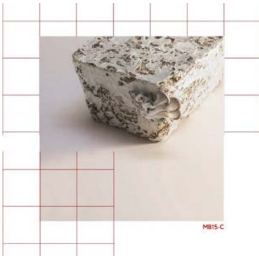
Fig.1 - The MB15-C brick, a mixture of sawdust and hemp. Some mushrooms grew, to show the living aspect of mycelium
