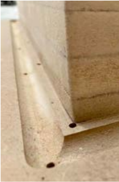
Fig.22 - A specific counter mold made to press the plastic mold for mycelium panels
