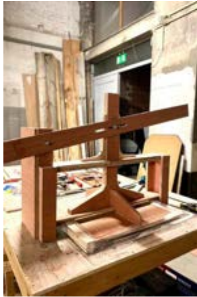
Fig.23 - The press to maintain substrates dense enough into the mold
