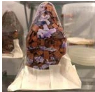
From top to down. Fig.6 - First step: the mycelium is fed and first grow in sterilized boxes...; Fig 7 Second step: ... before being inoculated into microperforated bags ; Fig 8. Third step: the mold is than sterilized, before inoculation
