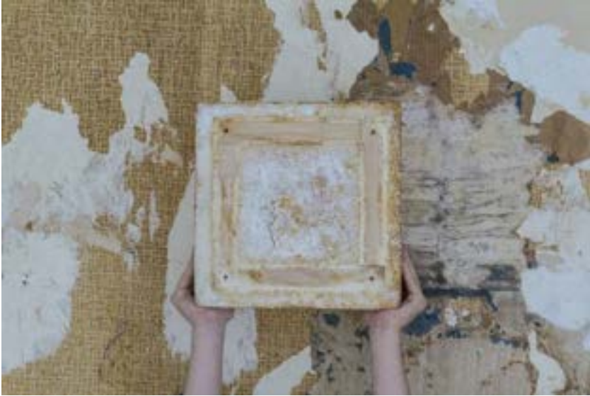
Fig 11. The mycelium grew into the mold, along "waiting woods", which are maintained by the mycelium. The wooden seat is then fixed into those waiting woods. It could be applied to prefabricated mycelium-based insulated wall.
